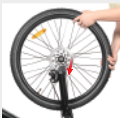
Put the wheel into the fork
