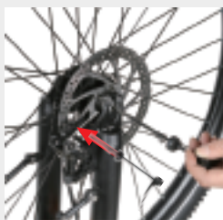
Place the quick release clamp into the front wheel clamp slot
