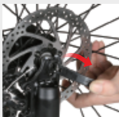
Press the quick release clamp firmly to ensure firm
