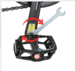
Tighten the right pedal "R" clockwise
