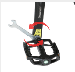
Tighten the left pedal "L" counter clockwise
